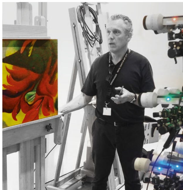
Properly conserving art for Dale Kronkright (right) means protecting art from vibrational stress during transportation. Here he is using a Polytec MPV-800 Multipoint Vibrometer system to analyze the vibrational characteristics of a painted canvas.
