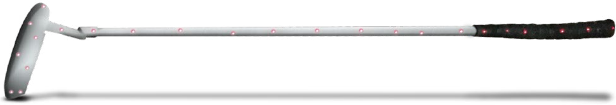
Figure 2: The putter that was tested is shown here with 24 laser measurement spots clearly visible.
