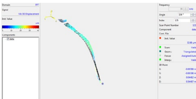
Figure 4: Deflection shape of the PS instrument during ultrasonic activation.
