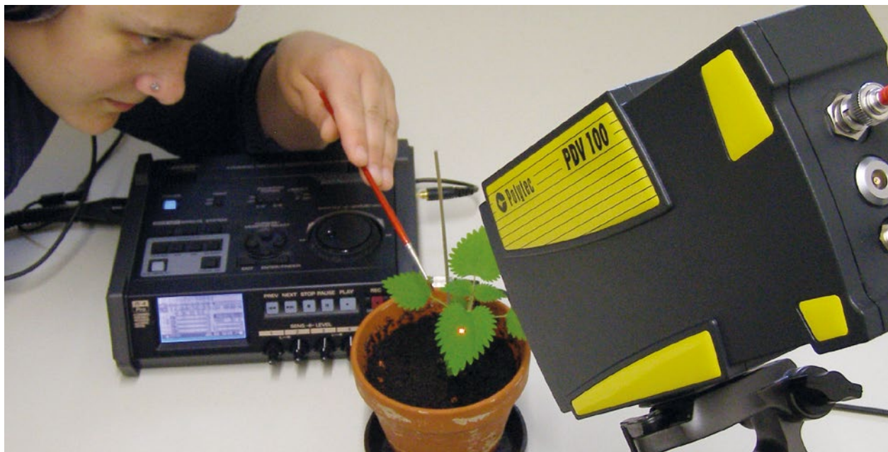
Figure 1: Experimental setup for recording planthopper songs. The vibrations are registered with a PDV-100 laser vibrometer either directly on the animal or on its host plant.
