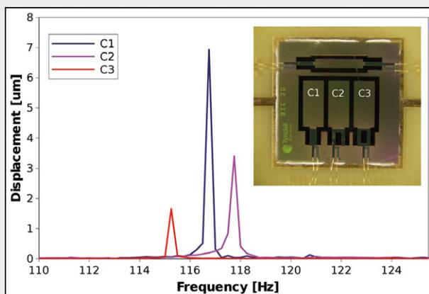
Figure 5: Resonance peaks measured by the vibrometer for three cantilever structures with slightly varying beam designs.
