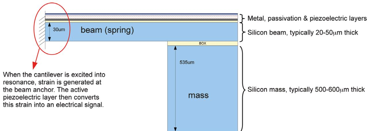
Figure 4: Schematic showing the cross-section of a silicon-based piezoelectric energy harvester.
