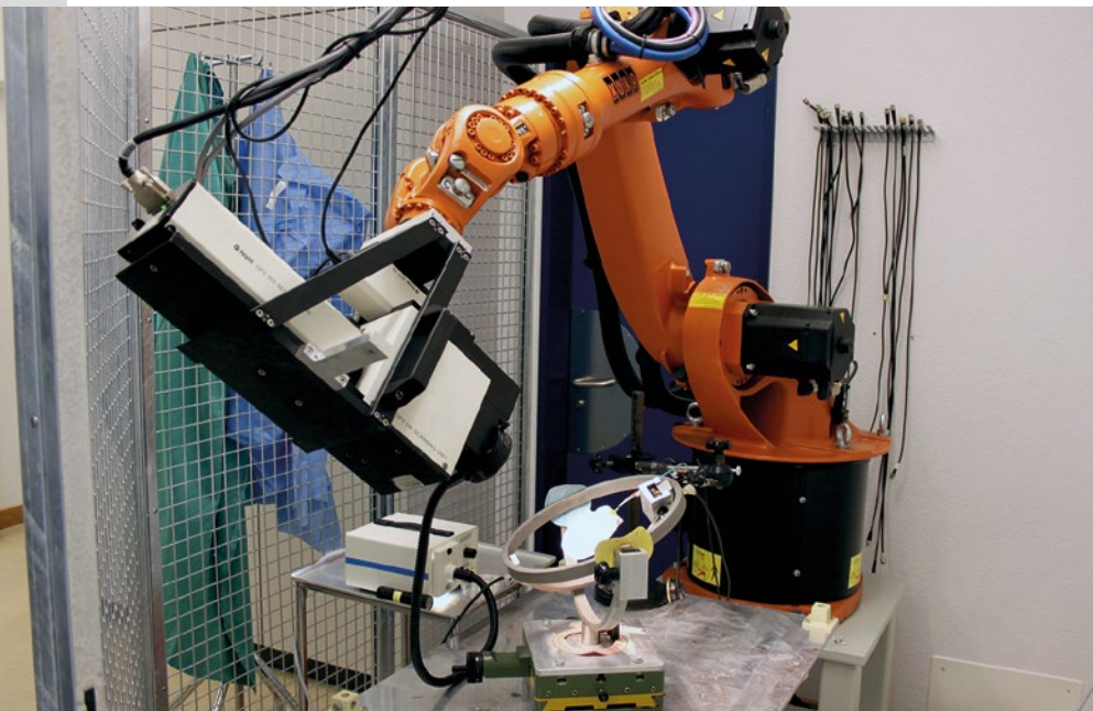
Figure 2: Experimental setup: the robot arm enables control of the desired position of the scanning-laser-vibrometer so that vibration of the stirrup can be measured as well as vibrations of the temporal bone.
