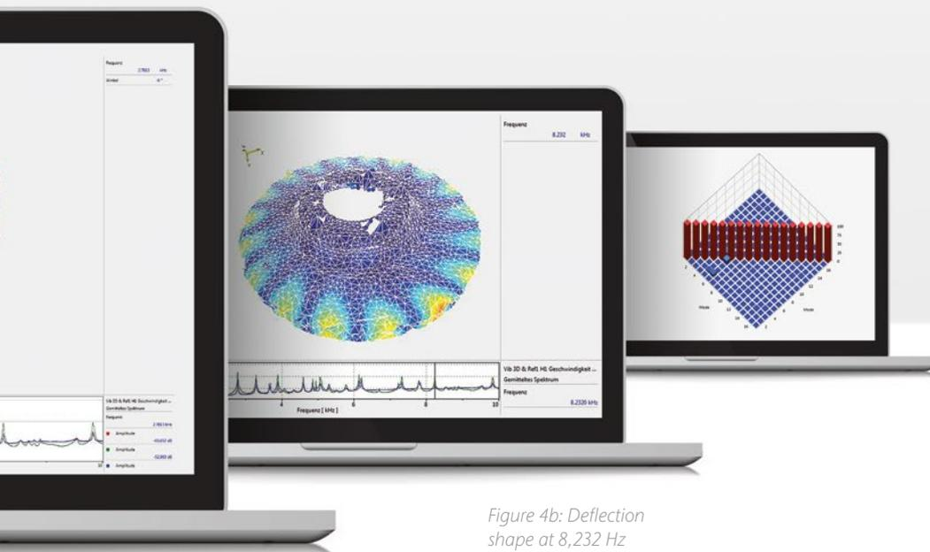
Figure 4b: Deflection shape at 8,232 Hz
