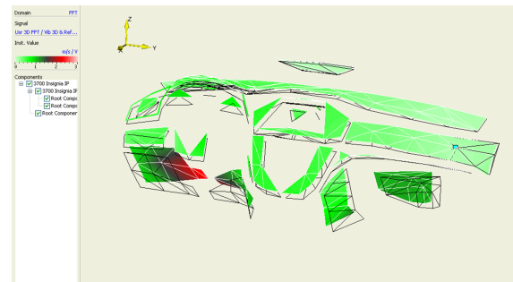
Figure 2: Operational deflection shapes of the instrument panel taken with the 3-D Scanning Vibrometer for modal correlation.
