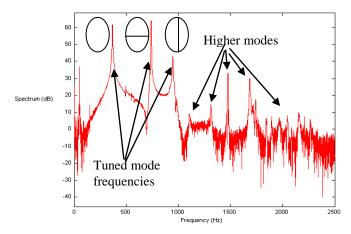
**Figure 6:** Typical frequency response spectrum for outer note on the soprano pan. First three modes are usually tuned into a nearly harmonic relationship. Higher modes are not harmonic but contribute to the overall timbre of the steelpan. Obtained using 1D scanning laser Dopler vibrometer and excitation using an impact hammer.
