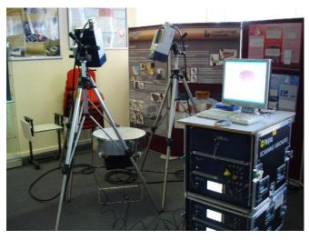
**Figure 3:** Set-up of the tri-laser system for the 3dimensional scans of soprano steelpan
