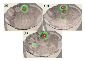
**Figure 4:** First three flexeural modes of C4<sup>#</sup> note region: (a) 276Hz, (b) 550Hz and (c) 640Hz
