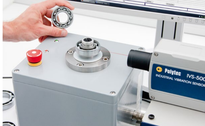
Ball bearing test bench with an IVS-500 Industrial Vibration Sensor
