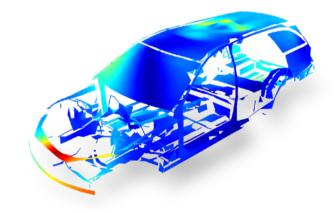
Testing time for structural analysis of complex shaped objects like complete vehicles is drastically reduced from weeks to only a few hours and is conducted automatically overnight.
