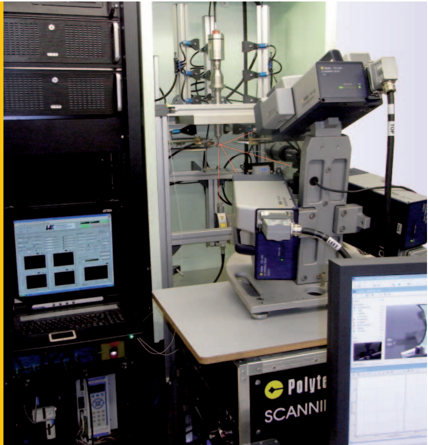
Fig. 1: Experimental setup for ultrasonic fatigue testing.
