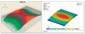
Fig. 3: First ODS measured at 20.9 Hz (left) corresponding to the simulated mode at 18.7 Hz (right).
