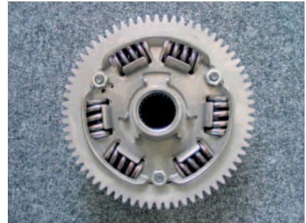
Fig. 8: Spring package for the clutch torsional vibration damper.
