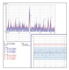
Fig. 2: Sideband energy measure based on order analysis for assessment of toothing vibrations.
