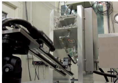
Fig. 2: Pre-validation of a valvetrain layout on a single-valve test bench.
