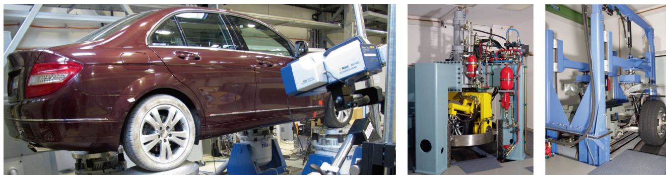
② Overview of the tyre testing environment at the Dresden research centre – vibration test stand at the Fraunhofer IWU (left), external drum test stand at the IAD (centre) and wheel suspension test stand at the IAD (right)
