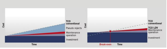
FIGURE 4 Comparison of the TCO using different measurement methods (left: TCO for conventional testing methods; right: TCO when using Laser Doppler Vibrometers (LDV)) (© Polytec)
