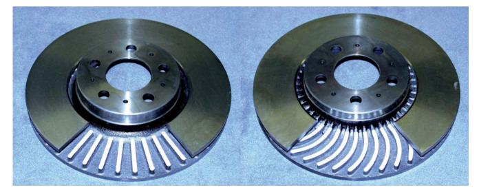
Figure 11: Structural imbalance due to modification of the disc stiffness (straight and bent cooling ducts)
