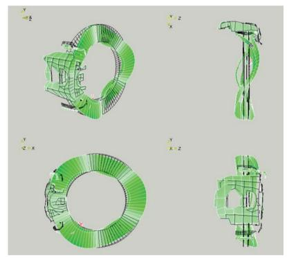
Figure 8: Measured operational deflection shapes
