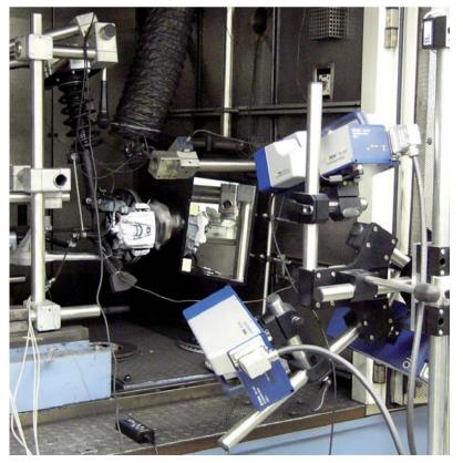
Figure 6: Brake system on the brake dynamometer [2]
