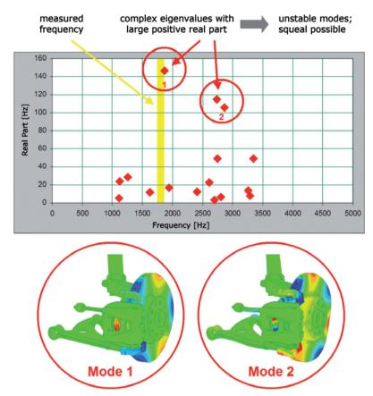
**Figure 3:** Two results of complex Eigen value analysis as modes 1 and 2 – only mode 1 at the measured frequency (yellow) leads to an audible squeal
