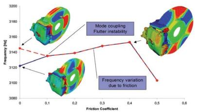
**Figure 9:** Emergence of squealing brakes due to mode coupling depending on frequency and friction coefficient
