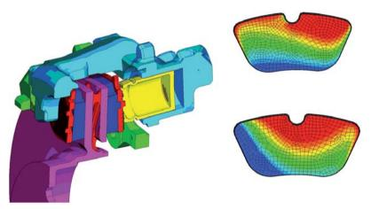
Figure 2: Presentation of the components (left) and calculation of deformation due to clamping and peripheral forces (right)
