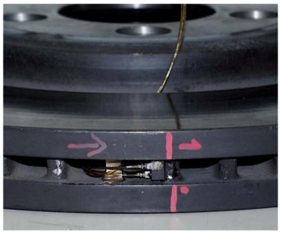
Figure 7: Brake disc with tri-axial accelerometer [4]
