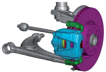
Figure 1: FE model of the brake system for complex Eigen value analysis
