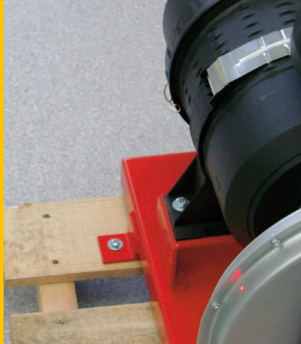
1 Non-contact vibration measurement by laser light on electric motors for acoustic tests
