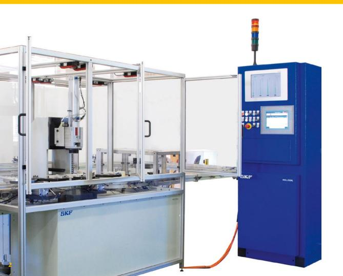
Inline noise tester for car wheel bearings (hub units)
