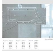
**4** Amplitude distribution on the surface of the sonotrode
