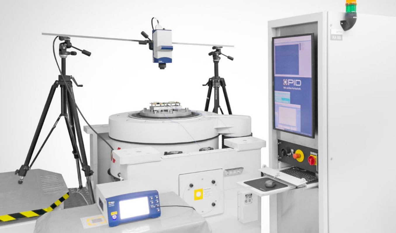
1 VibroFlex QTec®: shaker control for vibration testing of a power elec- tronics at PID test & engineering GmbH.
