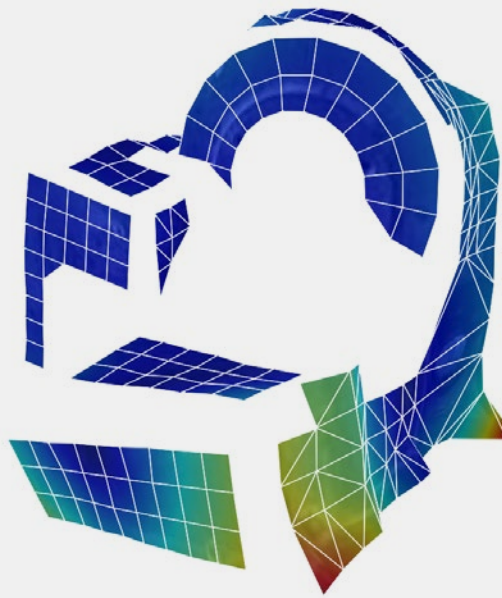
5 Deflection shape of the bell housing at 1102 Hz
