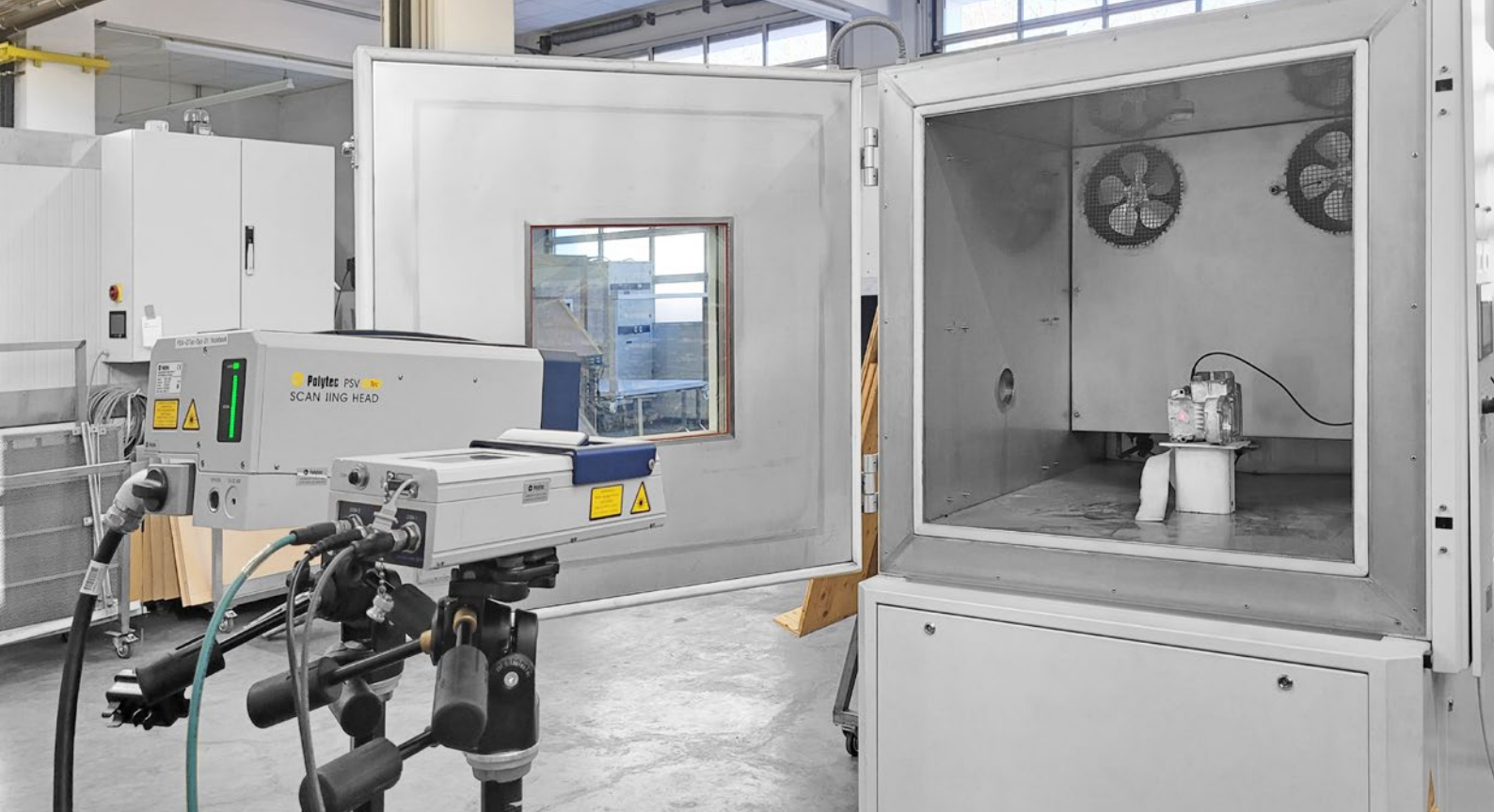
1 Measurement on gearbox bell housing inside a climate chamber with the door open using a QTec Scanning Vibrometer and a VibroGo
