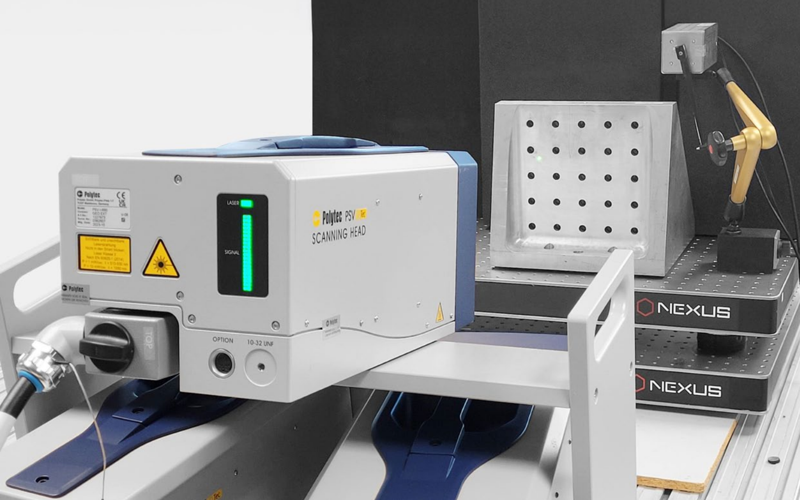
1 Test setup for resonance frequency determination using automated hammer excitation on a vibration-decoupled table. A Polytec QTec 3D scanning vibrometer can be seen in the foreground.
