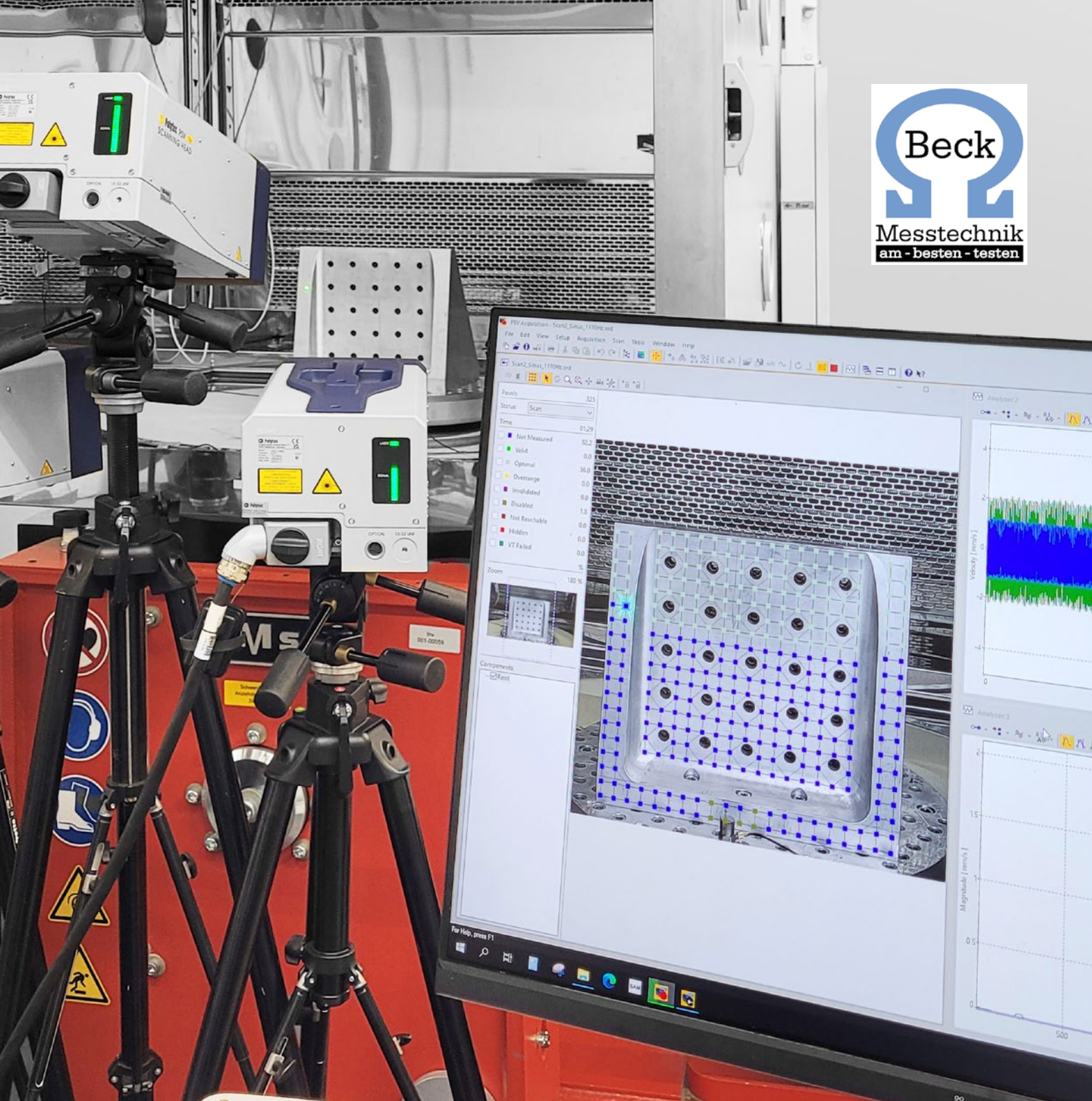
3 Test setup for experimental modal analysis using an electromechanical shaker at Beck-Messtechnik, a renowned measurement technology specialist for environmental simulation. A Qtec 3D scanning vibrometer can be seen next to the shaker. The PSV measurement and evaluation software is visible in the foreground.
