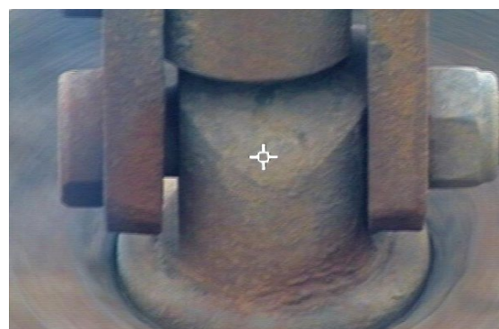
3 Measurement point with posi- tion of the laser beam in the video image of the RSV-150
