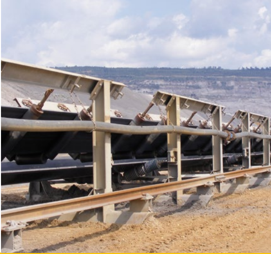
1 Conveyor belts for excavated material
