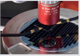
Figure 2: Scanning laser-Doppler vibrometer measurement of a single MEMS membrane on the wafer
