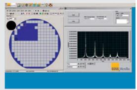
Figure 3: Wafer testing process and vibration signal displayed in the SUSS ProberBench™ Software
