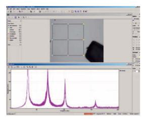
Figure 1: Measurement grid (top) and frequency spectrum (bottom) of the device displayed in the Polytec Scanning Vibrometer Software
