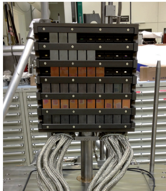
1 Sample holder with 6 different materials
