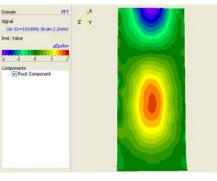
Fig. 5f) Strain along short axis at 18100 Hz with VideoTriangulation.
