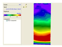
Fig. 4c) Strain along the long axis of the blade at 512 Hz without VideoTriangulation.
