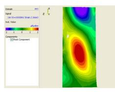
Fig. 5e) Strain along short axis at 18100 Hz without VideoTriangulation.
