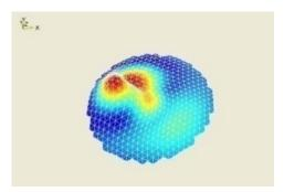
Fig. 3a) 3-D vibration at 102 kHz without VideoTriangulation.
