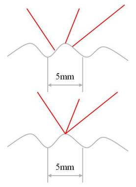
Fig. 1: beam intersection with standard 3-D coordinate measurement as compared to ideal case.
