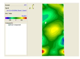
Fig. 5c) Strain along long axis at 18100 Hz without VideoTriangulation.
