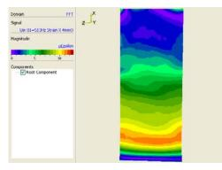
Fig. 4d) Strain along the long axis of the blade at 512 Hz with VideoTriangulation.
