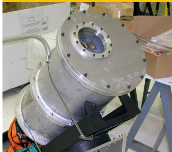
4 PSV Scanning Vibrometer in pressurized canister
