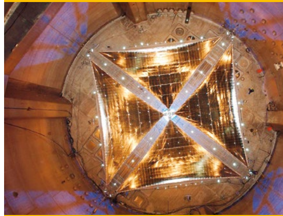
2 Deployed 20- meter solar sail on vacuum chamber floor
