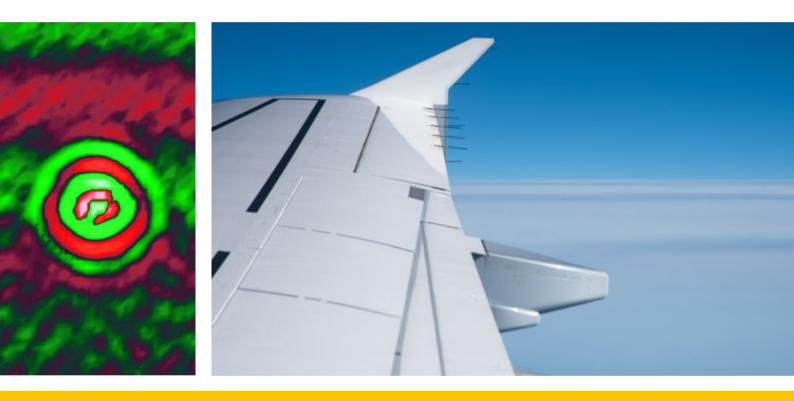
Aircraft Health Monitoring Laser Vibrometry for Damage Detection Using Lamb Waves Application Note
