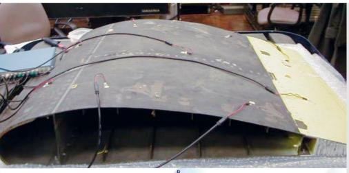
Measurement Setup: Piezoactors for local excitation of Lamb waves on a carbon fiber
