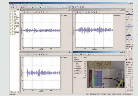
**2** In-plane and out-of-plane Lamb wave responses plotted using Polytec's PSV Software 1
