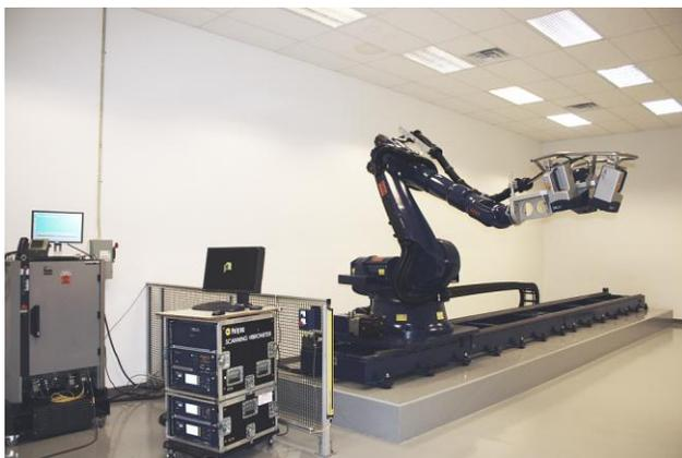
**Figure 4: RoboVib Test Cell**
