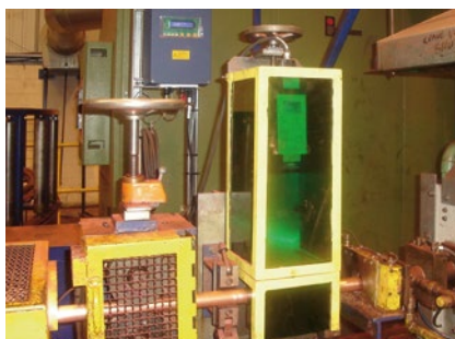
Two of the installed LSV Laser Surface Velocimeters for cut-to-length control at Mueller Copper Tube in Bilston, Great Britain.
