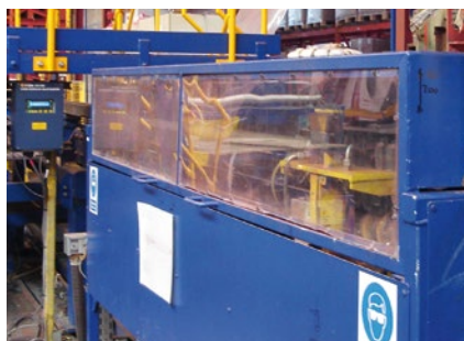
Two of the installed LSV Laser Surface Velocimeters for cut-to-length control at Mueller Copper Tube in Bilston, Great Britain.
