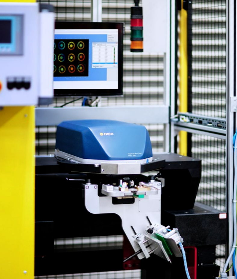
Figure 2: TopMap Pro.Surf sensor integrated into a production line
