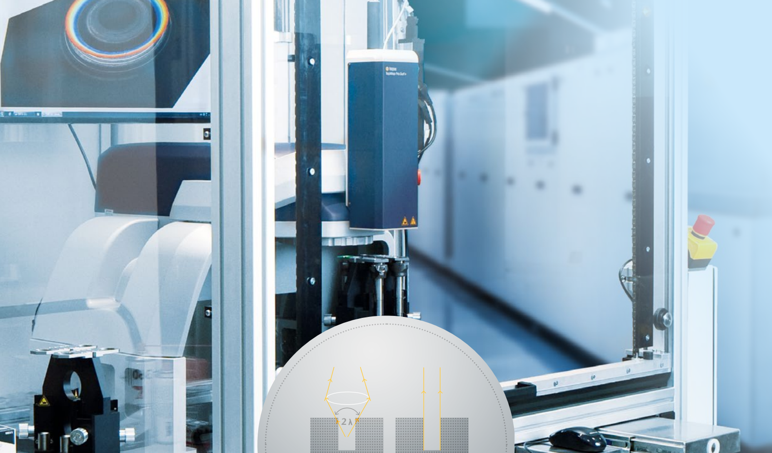
Figure 4: High aspect ratios can be easily characterized with telecentric optics used in Polytec large FoV systems
