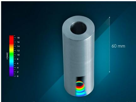
TopMap systems offer scan ranges of up to 70 mm – e.g. for measurements at the base of drilled holes. The telecentric light beam path avoids shadowing effects.
