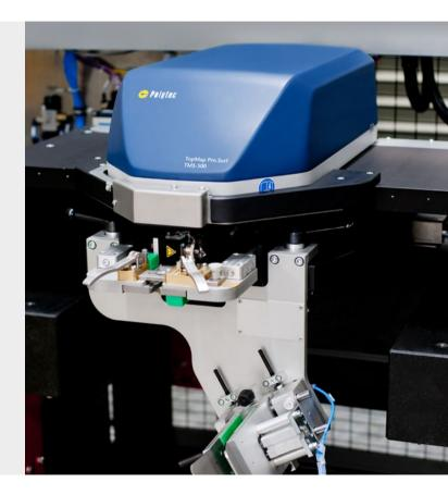
Sensor heads designed for machine integration: safe working distances and objective-free sensor design assure collision-free and smooth production processes.
