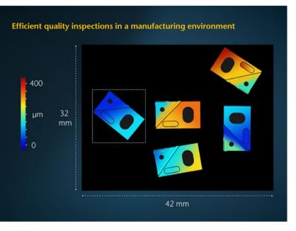
Automatic sample recognition (geometry and orientation) and the large field-of-view (FOV) allow quick and efficient multi-sample measurements without mechanical fixture.
