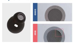
Earphone Filter Mesh Inspection Classify 6 types of filter mesh including regular items and defective items such as broken yarn
