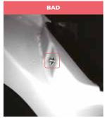
Bolt and Nut Assembly Status Inspection Check an assembled state of bolts and nuts using Object Detection model
