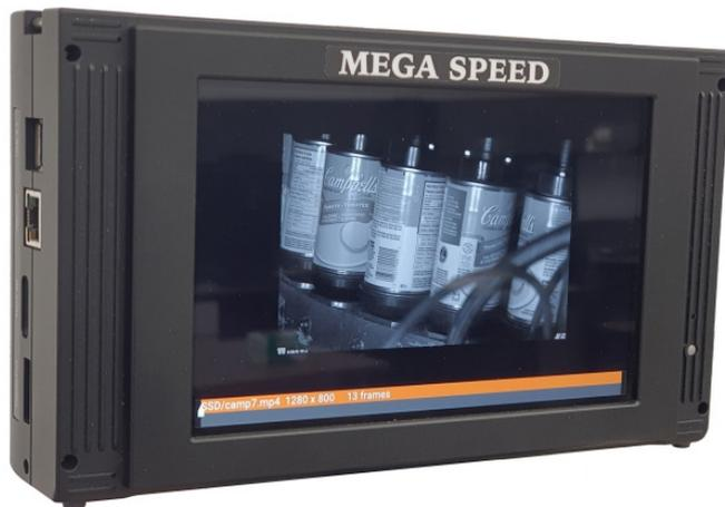
New from Mega Speed Corporation the Mega Speed Max V1 with Direct-To-Drive recording technology which in many applications eliminates the need for traditional record/save cycles found in most other high speed cameras.
