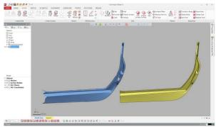
The SMARTTECH 3D scanner was used to obtain the geometry of the existing part, after it was fixed, to create an accurate CAD model. Thanks to the sharp angle between the camera and the projector SMARTTECH 3D scanners were able to scan the desired surface as it was installed on the car body with all limitations of the surrounding space.
