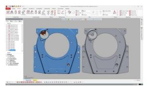
The clutch housing, weighing 12 kg and half-metre in length, was covered with an easily removable antiglare agent due to its glossy surface. The measurement was taken using the rotary stage and a MICRON3D scanner with an accuracy of 0.1 mm. It means that the virtual model might be different from the original not more than 0.1 mm, which was within the Arrinera's specified requirements.
