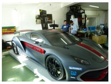
Arrinera is using a MICRON 3D scanner with the field of view of 800 x 600 mm and the resolution of 5 MPix. This cost effective 3D scanner helps them in designing, adjusting and inspecting their prototypes.
