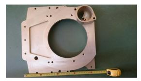
The SMARTTECH 3D scanner was used to accurately obtain the complete geometry of the object and to use it to design the desired component.
