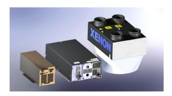
designed for providing unprecedented uniformity over a 12"x12" or 12" Diameter area. The system is designed to function as part of an integrated manufacturing system and provide controlled high peak power pulsed UV light. System interfacing is handled with low voltage I/O using a Programmable Logic Controller (PLC).
