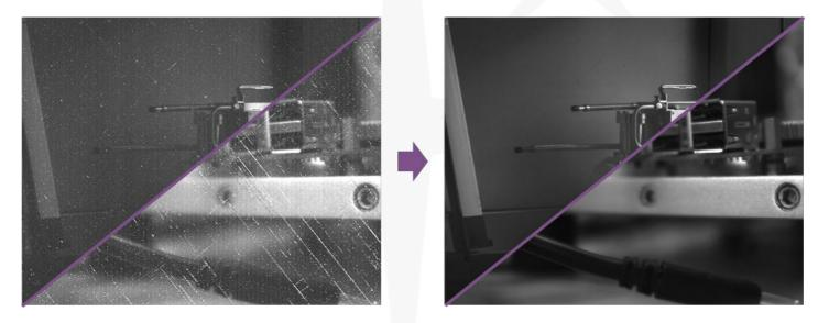
Images before and after applying the full correction process on a C-RED 2 ER 1.9µm (top) and a C-RED 2 ER 2.2 µm (bottom).
