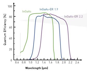
Comparison of the quantum efficiency curves for cameras based on standard InGaAs and extended range InGaAs (typical values).
