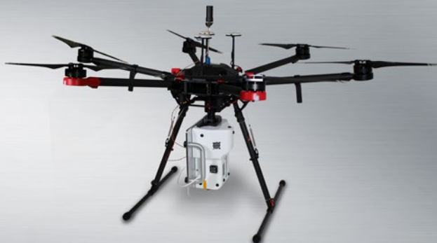
DJI M600 drone with broadband imager for 400 - 2,500 nm wave length
