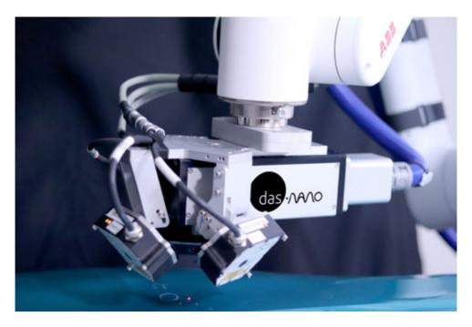
**das-Nano Irys** is a **contactless** patented system that using **terahertz waves** and proprietary algorithms developed by das-Nano provides the thickness of every layer in multilayer coatings in a non-destructive way.
