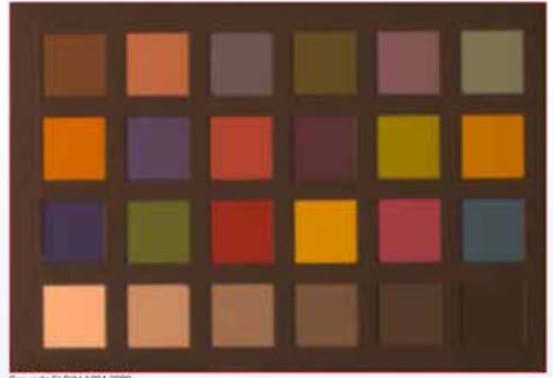
color checker illuminated with white LED
