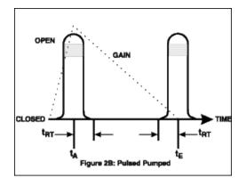
Figure 2: Driver Waveforms (not to scale)  $t_A$  = arrival time of pulse to be injected.  $t_E$  = time when circulating pulse is extracted.  $t_{RT}$  = cavity round trip transit time.
