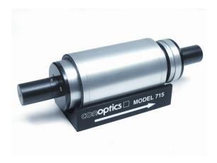
The Model 715-I is designed to work with unpolarized or randomly polarized lasers. The product replaces the conventional Glan polarizer's with calcite displacers at the input and output of the Faraday Rotator Assembly. Calcite crystals, when properly orientated, will generate two parallel beams with orthogonal polarizations.
