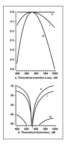
FIGURE 2: Insertion loss and extinction vs. wavelength (nm). I, uncompensated; II,  $0^{\circ}$  rotation compensated: III,  $90^{\circ}$  rotation compensated. Models 714 and 730,  $\lambda_0 = 880$ nm. Static losses are not included.
