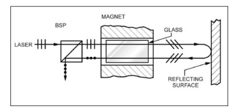
FIGURE 1: A basic optical isolator
