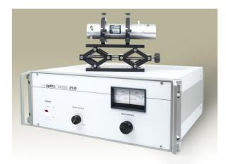
Conoptics series of electro-optic beam deflectors utilize a quadrapole electric field in an electro-optic material to produce a linear refractive index gradient proportional to the applied signal voltage. Choice of the proper material and crystallographic orientation eliminates piezoelectric ringing normally associated with other deflectors. There are no moving parts and they do not fatigue with prolonged use.
