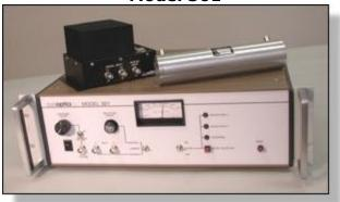
The system consists of a special version of the Model 311A Beam Deflector and a dual driver. This has been used for generation of auxiliary tracks in optical mastering equipment. The system accepts two inputs to generate analog and digital deflection.
