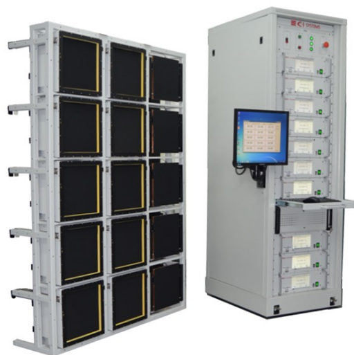
Figure 10: NUC Tower System with 15 controlled temperature blackbodies
