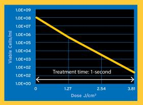
Destruction of B. subtilis in suspension exposed to Pulsed Light. Reduction of >6 log CFU/ml achieved within 1-second treatment time.
